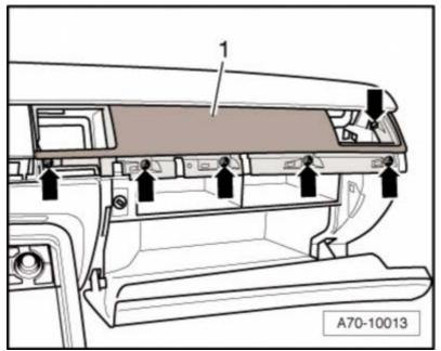
When you removed the bolts, detach the clip which is located at the left upper side. You can use a flat srew driver to pull up the plastic clip marked with the red arrow, while you can carefully start to pull the whole trim toward yourself. Be carefull do not brake it!
