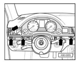
Hold the instrument cluster cover at the marked area, and pull it carefully toward yourself around 2-3cm as you can see the second picture! Just enough to make space for the MMI unit metal housing to get out.
