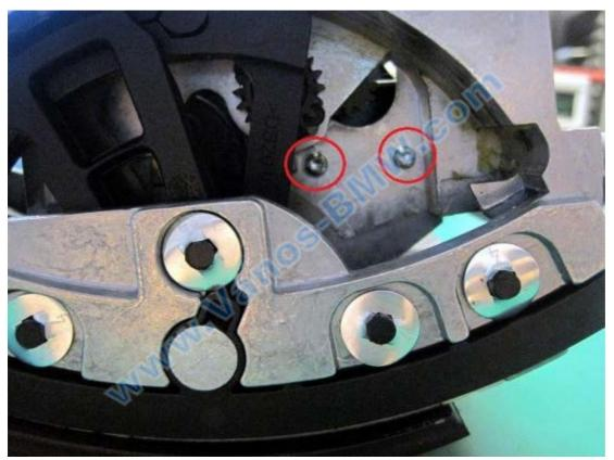
Remove the motor plastic gear, and install the new one. The original one was loosy, easy to remove, however the new one need quite a bit of force to install. Put the gear to the axis, and insert it to the table, and push the motor down in the arrow direction!
